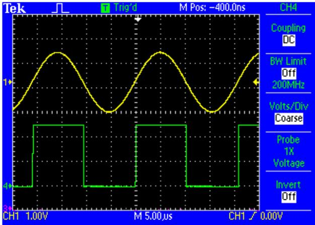
This snapshot shows a 10 MHz sine wave from a typical GPS receiver, converted into a TTL square wave.
