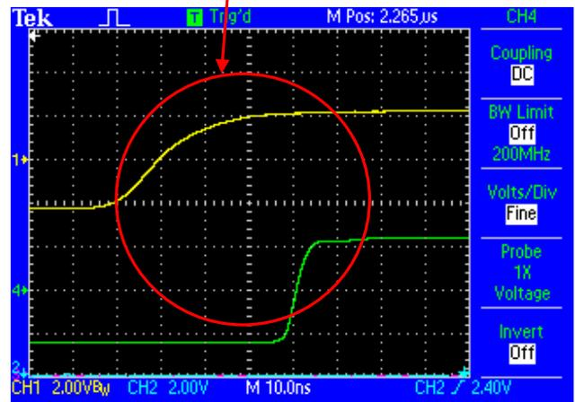
A closer look at the area of interest shows that the time delay (latency) is slightly longer in AES3id mode than in TTL mode, i.e. 30 nsec versus 25 nsec. The overshoot is optimized in AES3id mode, with a slight penalty in bandwidth. The rise time is 5 nsec in AES3id mode, as opposed to 3 nsec in TTL (clock) mode.
