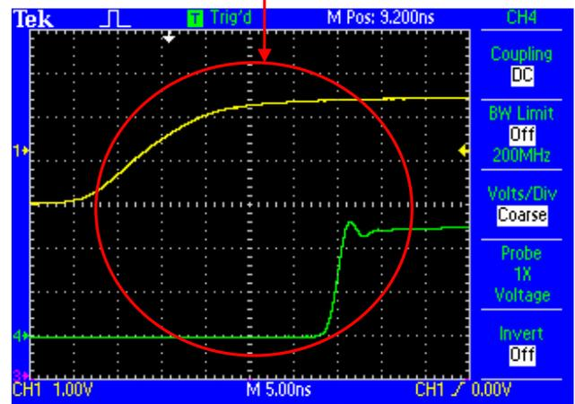
It can be seen from the magnification that the time delay (latency) of the unit is approx. 25 nsec when it is running in clock mode. Also, there is some cable ringing of approx 5%. The measurement was made with 10 m standard 68pF/m cable, terminated with 75 ohms.
