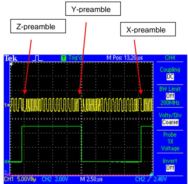
The extraction is done in the middle of the "safe window" where a clear definition exists between which audio data belongs to the low part of the word clock, and which audio data belongs to the high part of the word clock.
