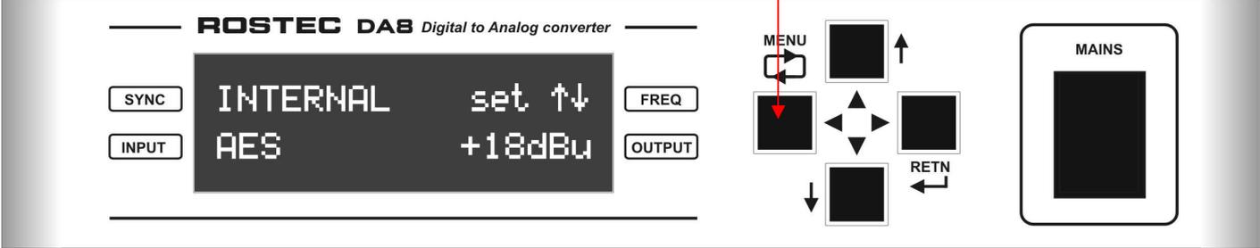
Step 3: Press one of the ARROW buttons. It doesn't matter which one.
